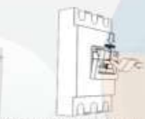
STEP - 2: - Fix the lockout on the circuit breaker, clockwise tighten the back button screw and afterwards close the red lockout handle
